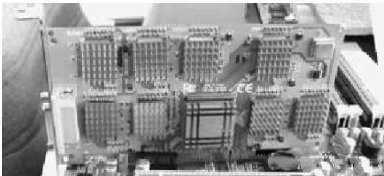
figure 3: PCI E-1X interface card insert into the PCI-E 1X slot
